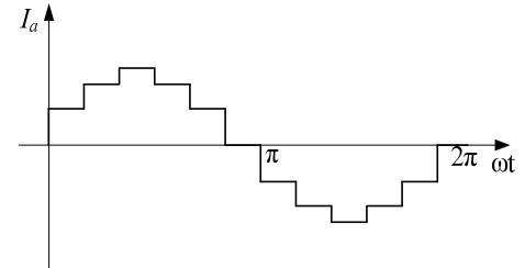
Fig. 6. Diagram of input current  $I_a$ .
