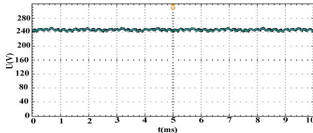
Fig. 20. Output DC voltage ( $K_u=0.9$ , Experiment).
