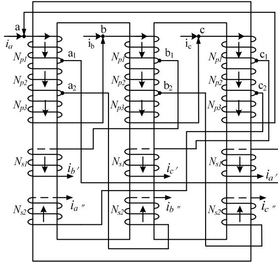
Fig. 7. Auto-transformer winding configuration of working mode 2.
