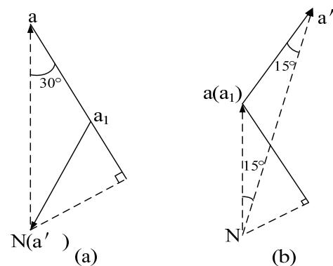
Fig. 4. Vector diagrams of  $U_{a'N}$  in limiting cases.
