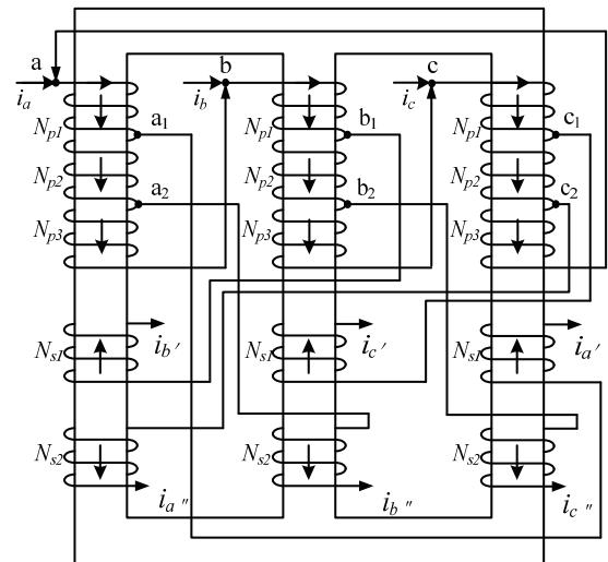
Fig. 5. Auto-transformer winding configuration of working mode 1.
