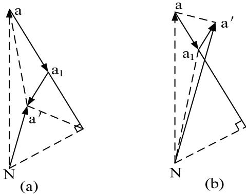
Fig. 3. Vector diagrams of output voltage  $U_{a'N}$ .
