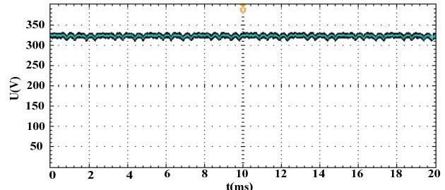
Fig. 22. Output DC voltage ( $K_u=1.2$ , Experiment).
