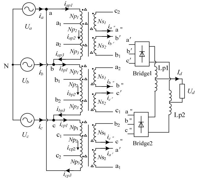
Fig. 1. Topology of step-down and step-up 12 pulse ATRU.
