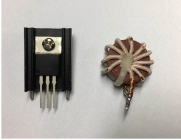
Fig. 9. Size comparison between a magamp and a MOSFET.
