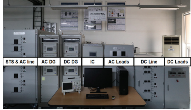
Fig. 18. Experimental setup based on VDER-HILS.
