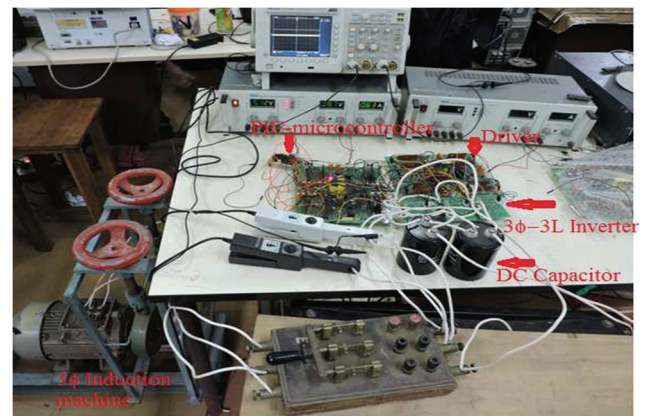
Fig. 13. Experimental setup of the three phase three-level SVPWM-controlled VSI.
