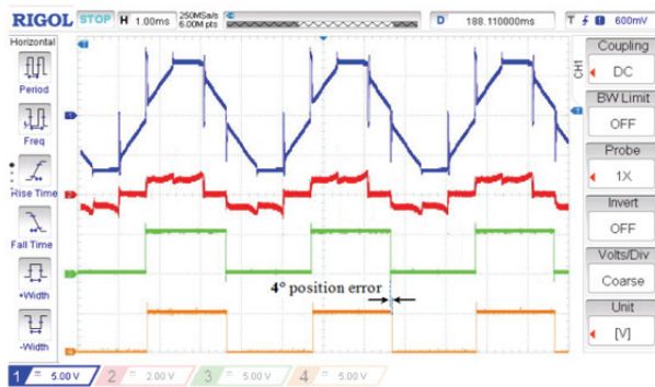
Fig. 22. Experimental waveforms obtained using the proposed method at a speed of 15000 rpm (from top to bottom): line voltage (5 V/div), phase current (2 A/div), IHS, and VHS.
