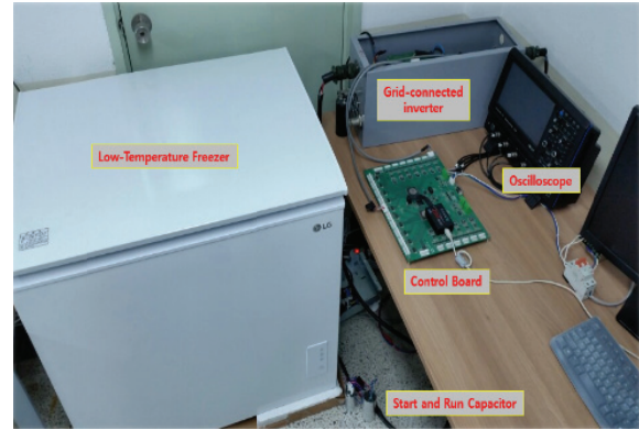
Fig. 10. Photograph of the experimental ultra-low temperature freezer using a SPIM driving system.
