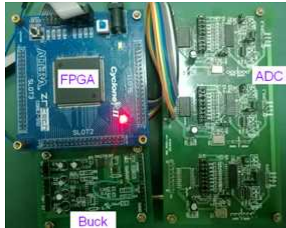
Fig. 11. A buck converter prototype and control system (FPGA+ADC).
