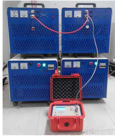
Fig. 12. Photo of a 40 kW transmitter.
