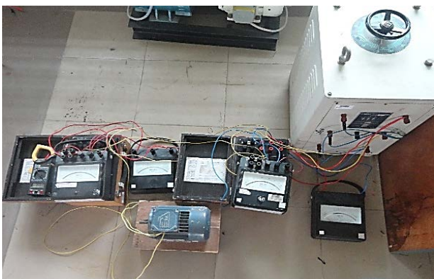
Fig. 16. Conventional test to estimate the motor parameters.
