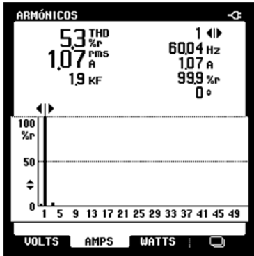
Fig. 10. SVPWM experimental THD current without the capacitor voltage algorithm.
