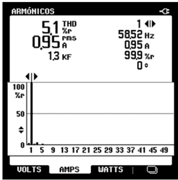
Fig. 9. SVPWM experimental THD current obtained the capacitor voltage-balancing algorithm.
