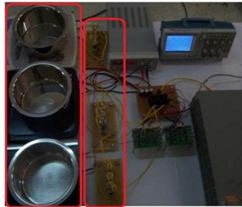
Induction heating loads Resonant capacitors
