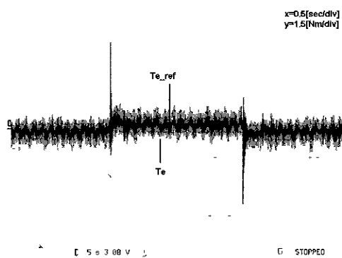
(b) Torque response characteristics
