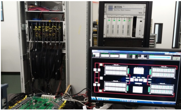
Fig. 15. RTDS simulation set for the proposed PSC PWM.
