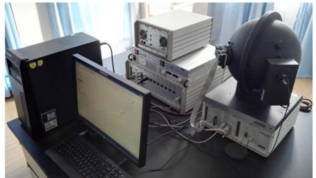
Fig. 1. Joint test system of TeraLED-T3ster equipment.
