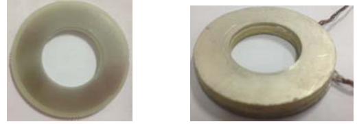
(a) LC unit. (b) CM and DM capacitor. Fig. 16. Basic unit of the EMI filter.
