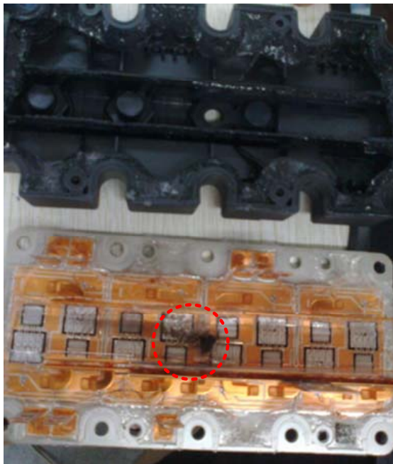
Fig. 19. Damage anatomy of power device caused by heat accumulation.
