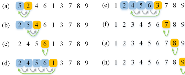
Fig. 11. Operations (a)-(h) of insertion sort on the array = \{5, 2, 4, 6, 1, 3, 7, 8, 9\} .
