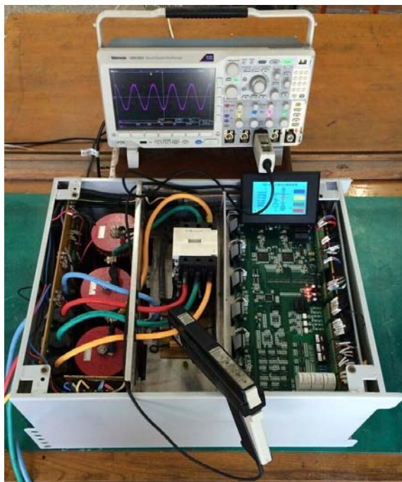
Fig. 10. Experimental prototype of the L -filtered grid-connected converter.
