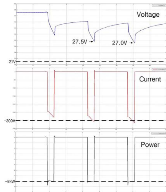
Fig. 11 Cold cranking test results of the HESS
