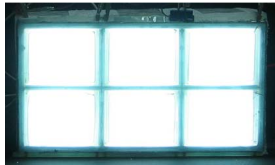
Fig. 5 A photo of 6-cell MFFL in stable glow discharge
