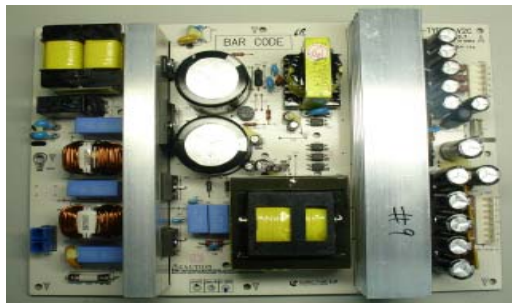
Fig. 10 Photograph of 385W LLC resonant converter
