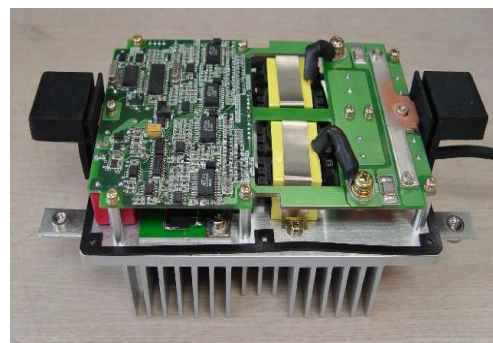
(a) 700W prototype with heat sink
