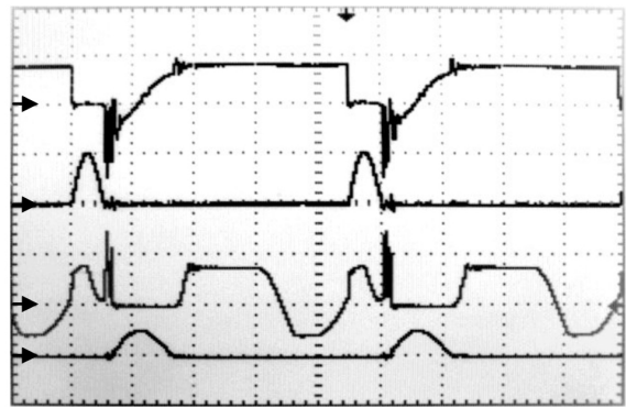
Fig. 4. Switching operation of HL-SwRC, respectively from top: V_{CE} of Q_2 , I_c of Q_2 , V_{CE} of Q_1 , and I_C of Q_1 . Scales: 2\mu\text{s}/\text{div} , 20\text{A}/\text{div} , 200\text{V}/\text{div} .
