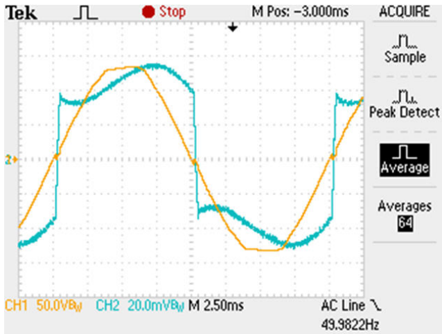
Fig. 8. Measured laboratory grid voltage and current (single phase controlled rectifier with inductive load).
