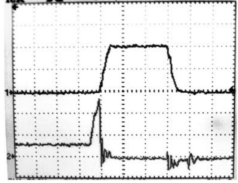
Fig. 7. Top: Sa1 voltage (50V/div), Bottom: Sa1 Current (4A/div), (time: 1μs/div).
