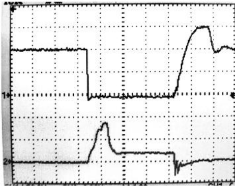
Fig. 8. Top: Sa2 voltage (50V/div), Bottom: Sa2 Current (2A/div), (time: 1 \mu s/div).
