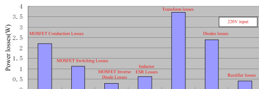
Fig. 17. Power-loss distribution of the studied converter.
