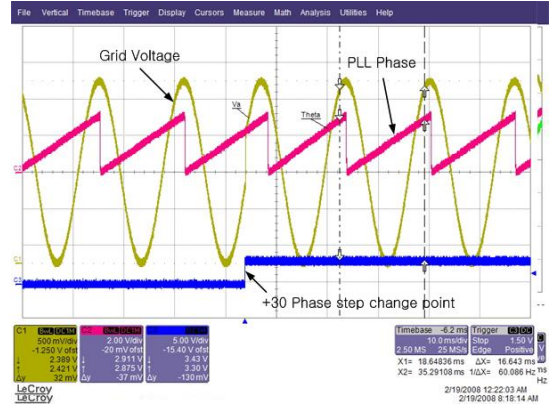
Fig. 14. +30 degree phase jump characteristics of the proposed PLL.
