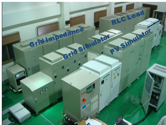
Fig. 17. Experimental equipment for PV PCS test.
