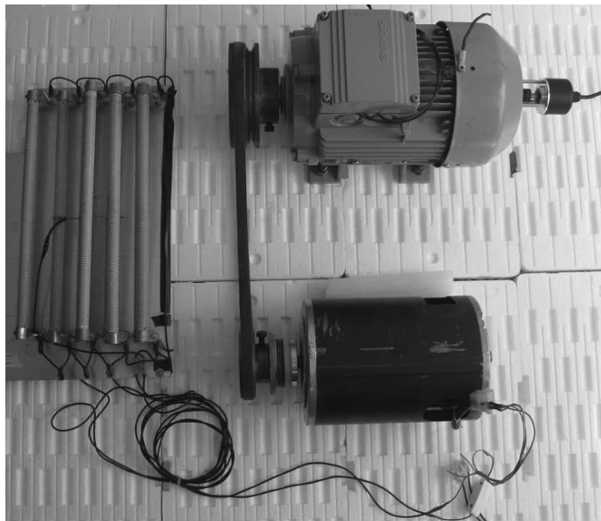
Fig. 17. DC generator as mechanical load.
