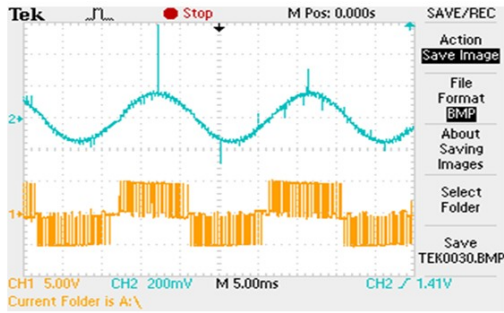
(a) Load voltage and current (scale:5ms/div,100v/div, 1A/div).
