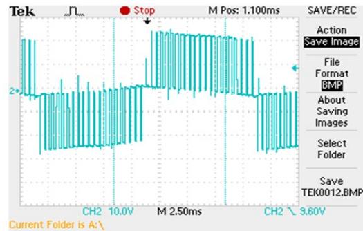
(a) Load voltage (scale:5ms/div,50v/div).
