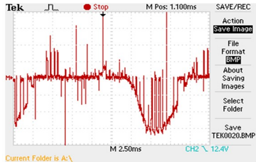
(e) Current in the other device (IGBT and diode) of a cell. (scale: 2.5ms/div,1A/div).
