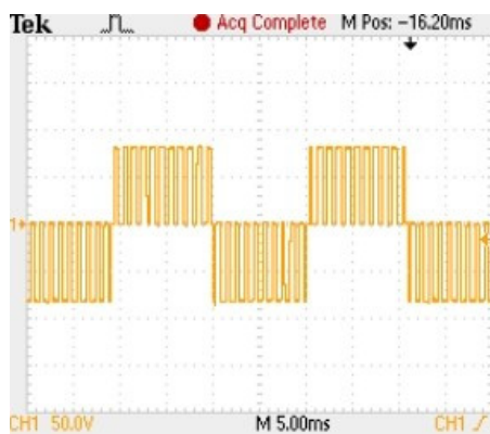
Fig. 22. Line-to-midpoint voltage at f_{sw} = 1\text{kHz} and m=0.8 ; 5ms/div, 50V/div.
