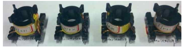
Fig. 16. Picture of the four tested transformers.
