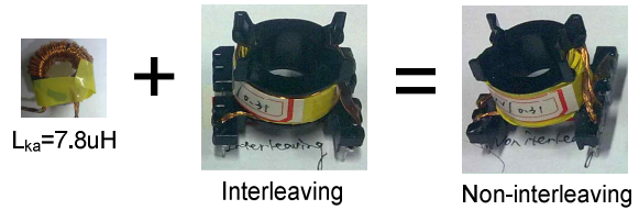
Fig. 17. External inductor L_{ka} to balance the leakage inductance.
