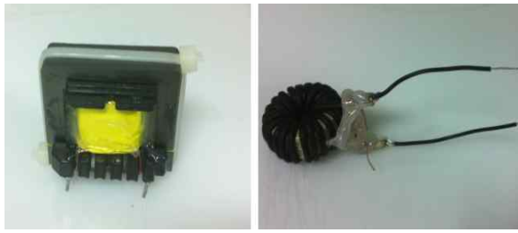
(a) Sandwich winding. (b) coaxial cable. Fig. 4 Sandwich and coaxial cable transformer.
