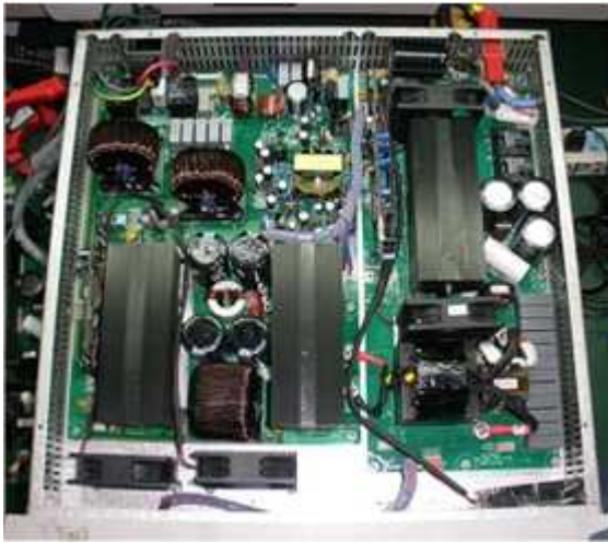
Fig. 15. 5-kW single-phase LCL grid-connected prototype.
