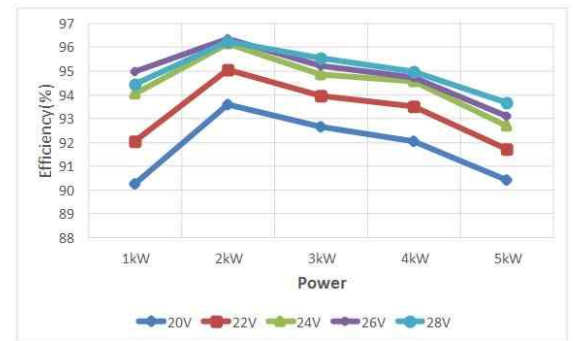
Fig. 22. Efficiency according to battery voltage, L_{r12} = 41.454 \mu\text{H} , f_s = 50 \text{ kHz} to 70 \text{ kHz} .
