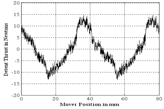
Fig. 1. Detent thrust versus position of PMLSM.
